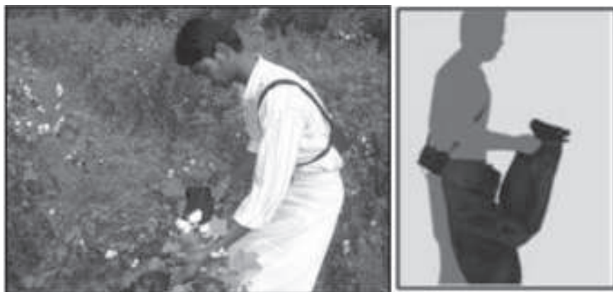
Fig. 4. Mounting of portable hand held cotton picker
