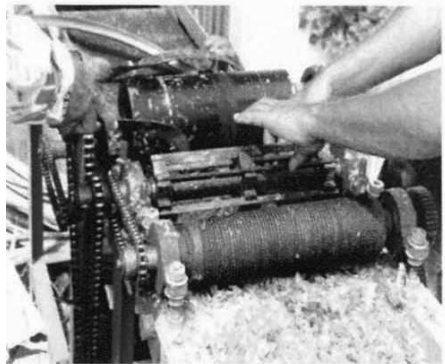
Fig. 9. Pineapple leaf fibre extractor
