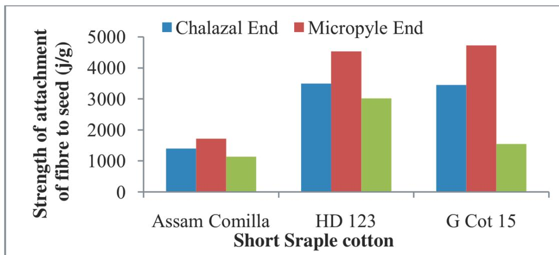
**Fig 7.**Strength of attachment of fibre to seed for short staple cotton
