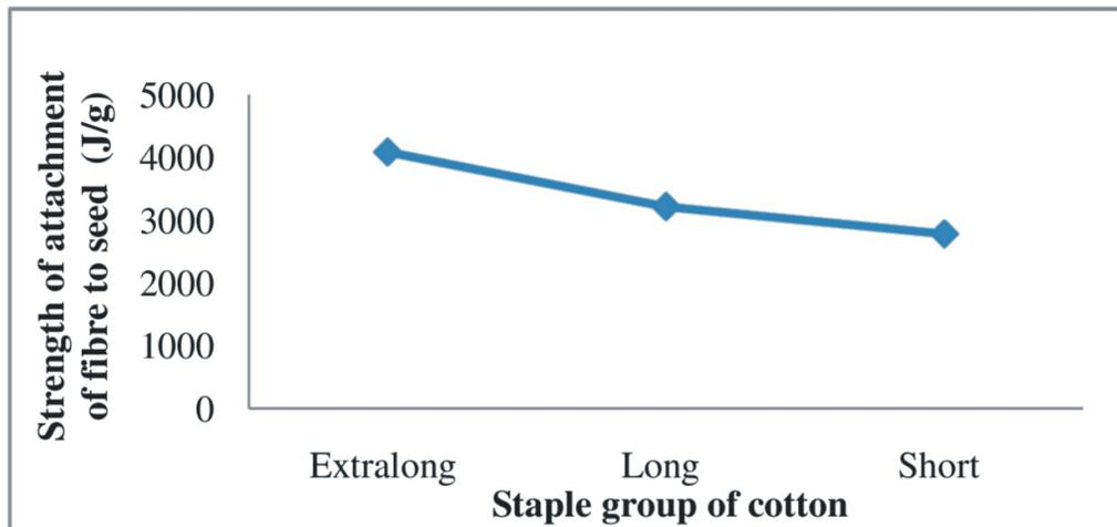
**Fig 8.** Effect of staple length on strength of attachment of fibre to seed
