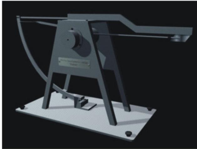
**Fig 1.** Cotton fibre seed attachment tester
