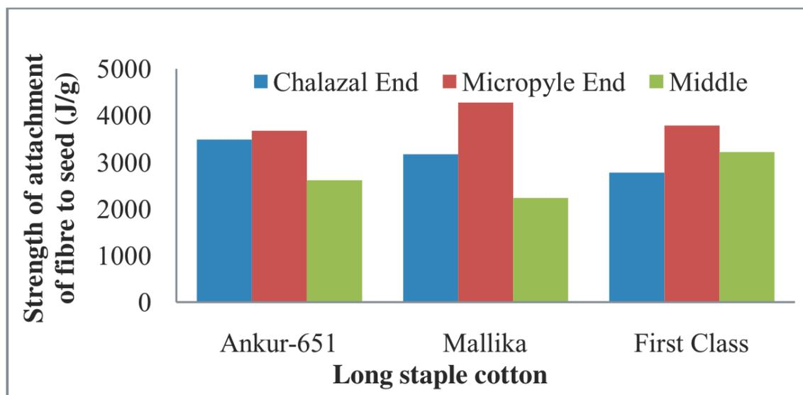
**Fig6.**Strength of attachment of fibre to seed for long staple cotton
