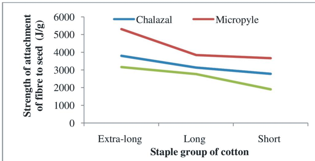
**Fig 9.** Strength of attachment of fibre to seed for different staple groups
