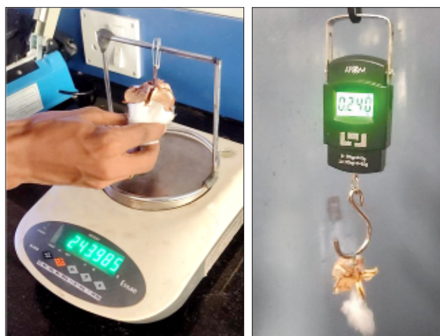
Fig. 2(a) & 2(b) Test setup for measurement of picking force
