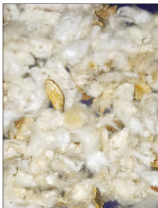
Fig. 2. Kawdi cotton with opened up fibres on passing through boll opener machine
