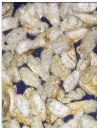
Fig. 1. Raw kawdi cotton showing closely held fibres unavailable for ginning
