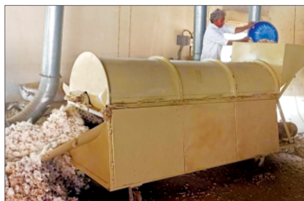
Fig. 6. Performance evaluation of new paddle type Boll Opener
