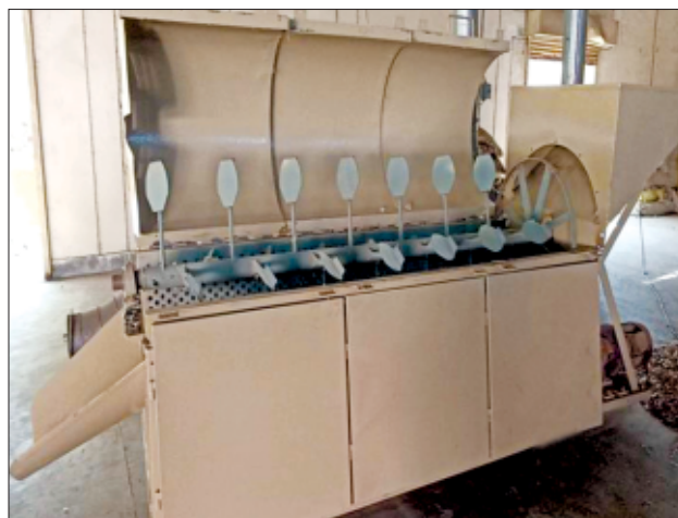
Fig. 4. Inside view of new paddle type boll opener showing beater assembly, motor drive, side mounted feed hopper, concave screen sections (12, 16 and 20 mm) and outlet chute
