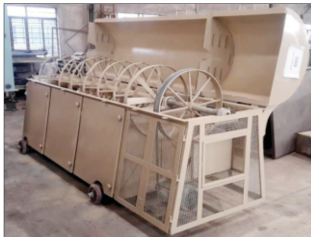
Fig. 3. Inside view of Bajaj Boll Opener showing helical beater type assembly
